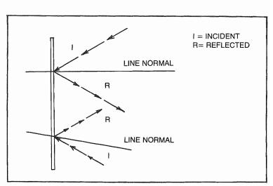
Fig. 4-1. A flat mirror. The line normal lies at a right angle to the plane.
