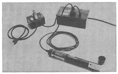
Fig. 10-11. Coherent CR-135 helium-neon laser. (Photo courtesy of Coherent Laser Division.)
