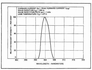
Fig. G-14. Typical spectral emission characteristic for a GaAs laser diode.
