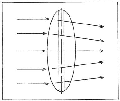
Fig. 4-14. Converging effect on a convex lens.
