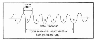
Fig. 2-3. This electromagnetic wavelength travelled 186,000 miles in one second.
