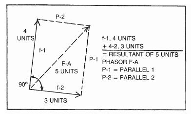
Fig. 9-2. Resultant of a phasor parallelogram.
