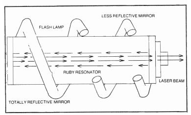
Fig. 6-2. An elementary ruby laser and its components.
