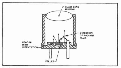
Fig. G-6. Schematic arrangement of a typical RCA IR-emitting diode mounted in an OP-17 package (scale exaggerated).
