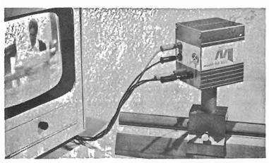
Fig. 5-15. Battery-operated, solid-state photodetector and amplifier with choice of ordinary or high power outputs can act as a receiver for the beam of a modulated laser to produce an audio output when connected to an oscil-loscope;..or TV picture when connected to a closed circuit monitor. (Photo courtesy of Coherent Laser Division.)
