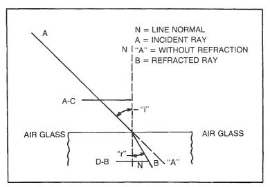
Fig. F-1. Angle of refraction.
