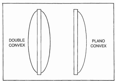
Fig. 4-13. Convex lens.
