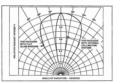
Fig. G-7. Typical radiant intensity patterns of RCA IR-emitting diodes.
