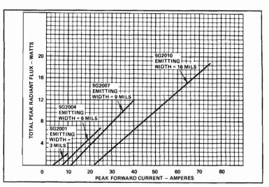
Fig. G-11. Typical peak radiant flux (power output) as a function of peak drive current.
