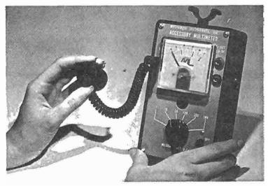
Fig. 5-13. Metrologic's 60-230 Photometer, in addition to being an excellent laser power meter at a very low cost, can also be used as a communications receiver. (Photo courtesy of Coherent Laser Division.)
