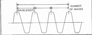
Fig. 2-2. A wavelength of 1 inch and a frequency of 4 Hz.
