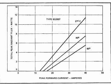
Fig. G-12. Typical peak radiant flux (power output) vs peak forward drive current showing the effect of temperature on threshold current.
