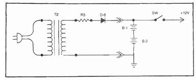
Fig. 8-3. Schematic for the battery charger.
