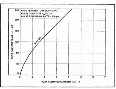
Fig. G-3. Typical peak radiant flux vs peak forward current.
