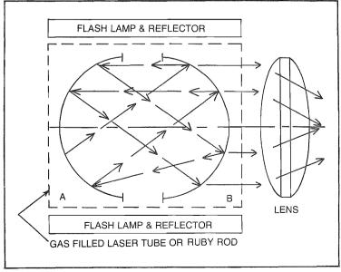
Fig. 4-10. Repetitive reflection as employed in a laser cavity.
