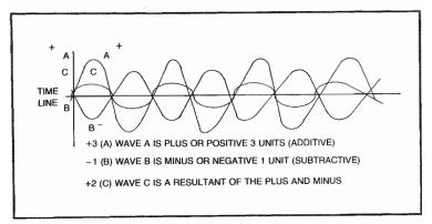
Fig. 2-8. Electromagnetic waves in exact out of phase subtractive superposition.
