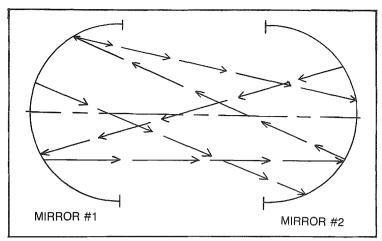
Fig 4-9. The repetitive reflection of two mirrors.
