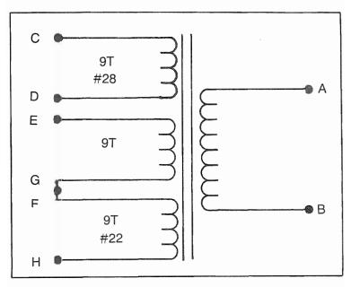
Fig. 8-4. Schematic for the square wave power transformer.
