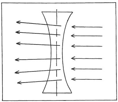
Fig. 4-15. Diverging effect on a concave lens.
