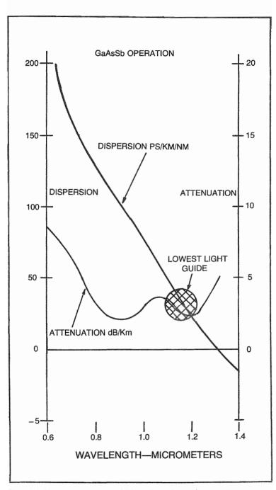
Fig. 11-1. Minimum loss chart exhibiting dispersion and attenuation.
