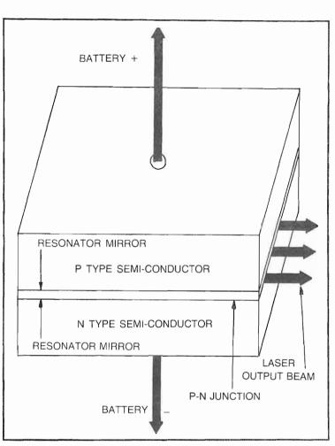
Fig. 6-4. A semi-conductor junction laser.
