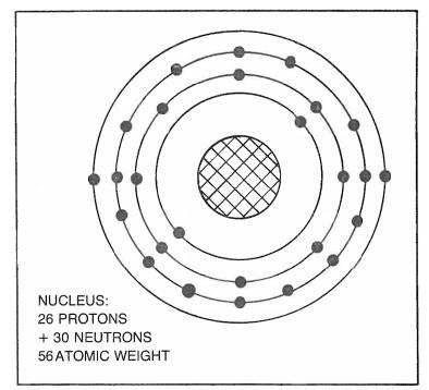
Fig. A-2. The atomic geometry of iron.
