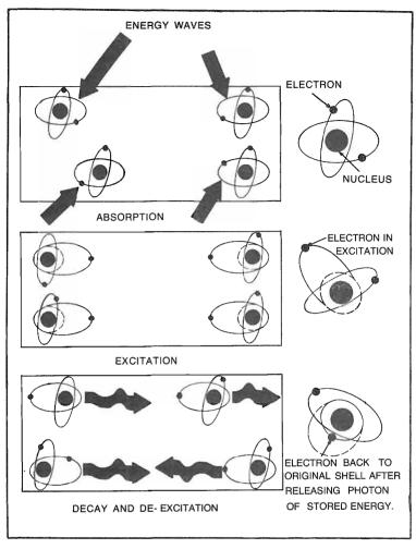
Fig. 1-3. Atoms and electrons go through absorption, excitation and decay in three separate environments.
