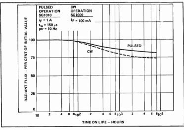
Fig. G-8. Typical life test data for RCA SG1009 and SG1010 IR-emitting diodes.
