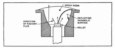
Fig. G-5. Schematic arrangement of a typical RCA IR-emitting diode mounted in an OP-10 package (scale exaggerated).
