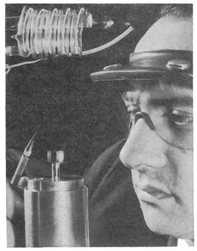
Fig. 5-2. This scientist views a cube of synthetic ruby crystal that forms the heart of a laser and generates the light. The light source (at top) is used to excite the tightly-packed atoms in the ruby which then amplify the laser's light into an intense parallel beam. (Photo courtesy of Hughes Aircraft Co.)
