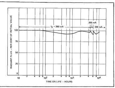
Fig. G-21. Typical life test data for a double-heterojunction AIGaAs laser diode type C30127.
