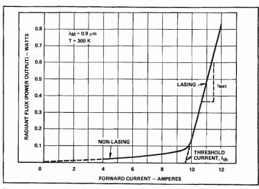
Fig. G-10. Radiant flux as a function of forward current for a typical injection laser diode.
