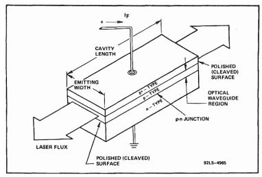
Fig. G-9. Typical injection laser diode structure.
