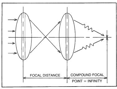
Fig. 4-18. The focal distance and compound focal point of two lenses.
