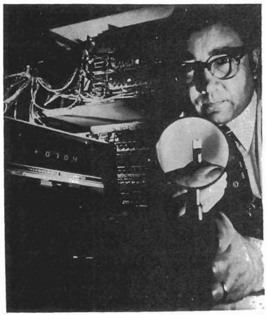
Fig. 5-10. A Bell Laboratories engineer exhibits a tiny solid-state laser perched atop a specially designed mount. Such lasers have average projected lifetimes of one million hours—about 100 years—at room temperature, according to the lab's accelerated-aging test results. (Photo courtesy of Bell Laboratories.)
