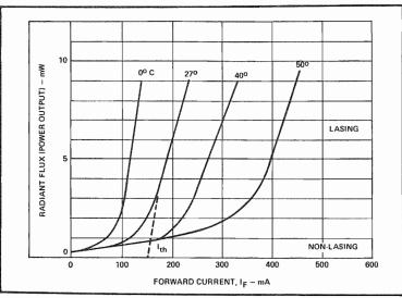
Fig. G-20. Typical radiant flux power output vs DC forward drive current showing the effect of temperature on threshold current.
